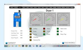
Indivdual machines can be monitored or operated from the TEXVIEW systems. e.g. for a Dryer, Input and output temperatures, drying times and alarms can be viewed.
