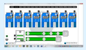
Overview of the dryer section behind a continuous batch washer, with the status of each dryer and location of the linen per customer.
